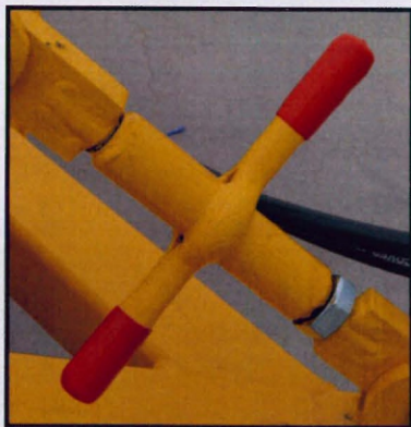
MOUNTED TURNBUCKLE ADJUSTS HITCH TO TRACTOR HEIGHT.
