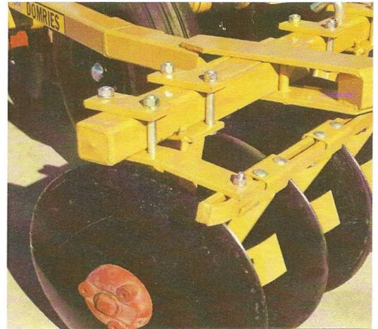
TRUNION TYPE SELF ALIGNING BEARING UNIT MOUNTED WITH A RUGGED BRACKET AND CLAMP ASSEMBLY.
