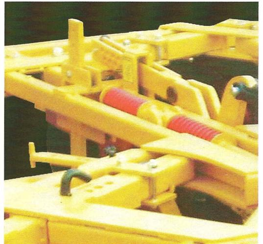
VIEW SHOW HEAVY 1X3 CENTER SHANK. SHOCK CUSHIONING SPRINGS AND DEPTH CONTROL SET BAR WITH TRANSPORT PIN.
