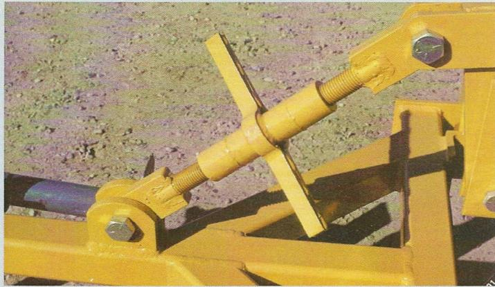
TRUNBUCKLE LEVELS THE MACHINE TO THE TRACTOR HITCH. THE MACHINE WILL REMAIN LEVEL THRU ALL LIFTING STAGES.
