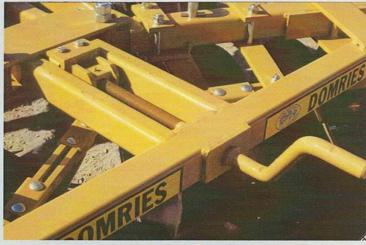
FINE TUNE CRANK CONTROL OF REAR GANGS TO ASSURE A FLAT AND SMOOTH FINISH.
