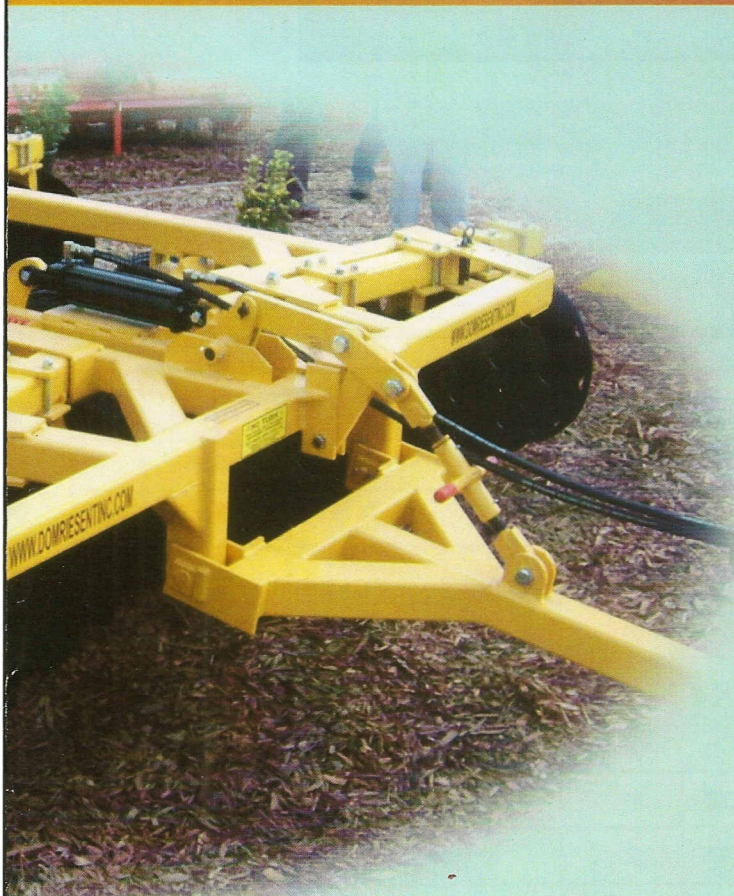
DEPTH CONTROL SET BAR WITH TRANSPORT SAFETY PIN IN PLACE. OPTIONAL CENTER SHANK AND SWEEP.
