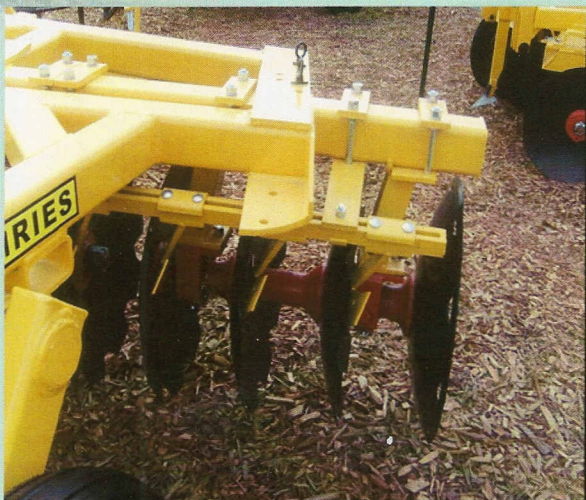
FRONT GANG ANGLE IS TYPICAL OF DOMRIES QUICK PULL PIN SETTING. POSITIVE MATCHED ANGLES WITH NON SLIP GANG SET PINS. NO WRENCHES NEEDED.
