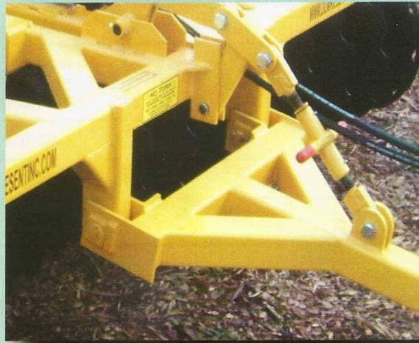
FRONT MOUNTED TURNBUCKLE ADJUSTS MACHINE LEVEL TO TRACTOR HITCH HEIGHT. LINKAGE WILL THEN KEEP MACHINE AT THE SAME LEVEL FROM DISCING TO TRANSPORT.
