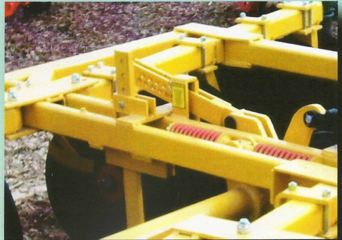
DEPTH CONTROL SET BAR WITH TRANSPORT SAFETY PIN IN PLACE. OPTIONAL CENTER SHANK AND SWEEP.
