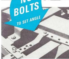
FOR INSTANT GANG ANGLE SETTING . PULL A PIN AND SET . NO SLIP OF BOLTS . POSI-TIVE PIN-IN HOLD SETTING . NO GUESSING OF ANGLE . COUNT THE HOLES AND SET
