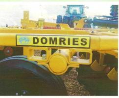
HEAVY DUTY AXEL SHAFT WITH 4 LUBRICATABLE BEARINGS.
