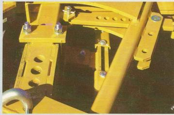
DROP PIN SET BAR FOR QUICK AND NON-SLIP SET OF GANG ANGLE OF 12" TO 28"
