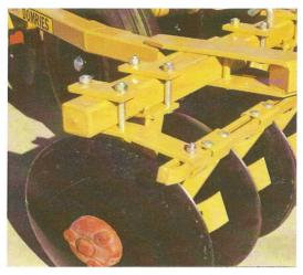
TRUNION TYPE SELF ALIGNING BEARING UNIT MOUNTED WITH A RUGGED BRACKET AND CLAMP ASSEMBLY.
