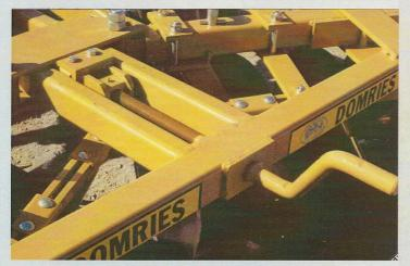
FINE TUNE CRANK CONTROL OF REAR GANGS TO ASSURE A FLAT AND SMOOTH FINISH.
