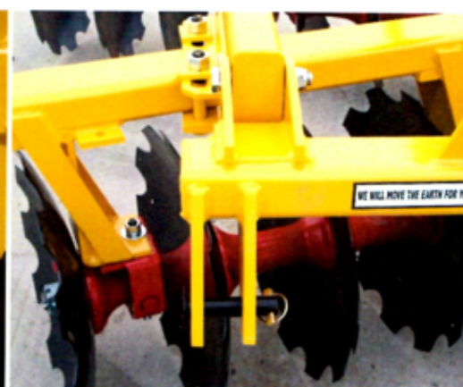
RUGGED HITCHING BAR HAS DRAFT CONTROL SELECTION
