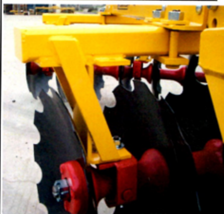
TRUNNION TYPE BEARINGS WITH STEEL PLATE FORGED BRACKETS.
