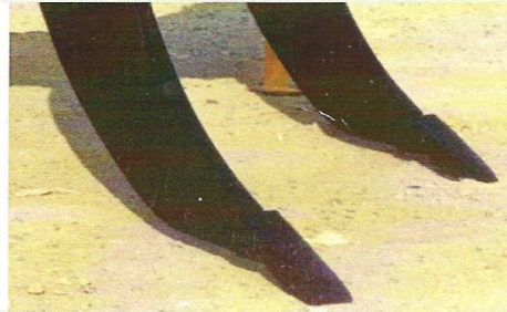
HI TENSILE STEEL REPLACEABLE SHINBAR PROLONGS THE LIFE OF THE SHANK.
