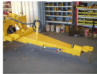
HITCH The long slender design of the hitch allows shorter turns behind dual wheel and track type tractors. The heavy wall tubing planted on both sides develops a super strong hitch needed for big H.P. tractors.
