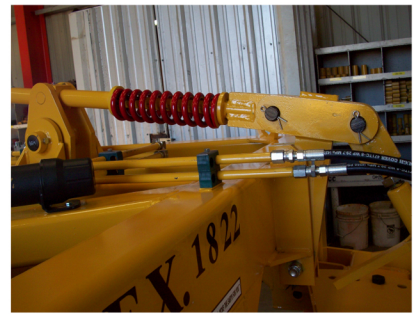
HITCH A series of holes allows fast offset adjustment. Front mounted turnbuckle adjusts machine level to tractor hitch
