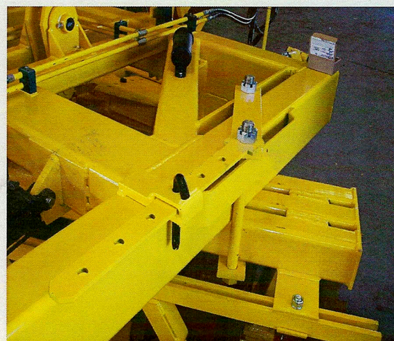
SET BARS USING TRACTOR POWER TO MOVE GANG BEAMS DROP SET PIN AT ANY ANGLE 16° TO 30° HANGER BOLTS GLIDE IN TWO CHANNELS ALLOWING AN EASY NON SLIP GANG ANGLE ADJUSTMENTS.
