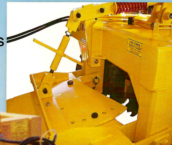
LEVELING LINKAGE IS PROTECTED AGAINST SHOCK WITH A HEAVY COMPRESSION SPRING. DRAFT TWO LEVEL HITCH HOOKUP.
