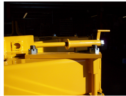
DEPTH CONTROL Threaded crank gives fine tuned depth of cut settings. A transport safety pin is also part of control unit.
