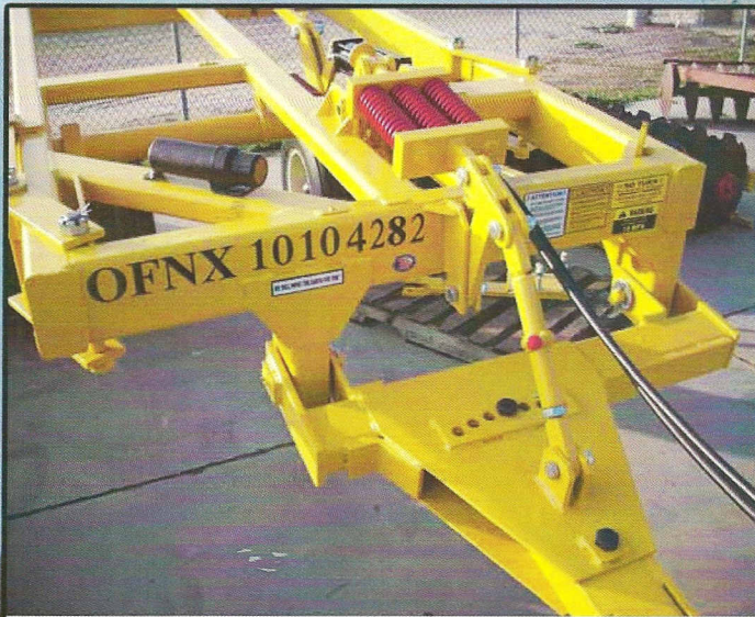
DUAL SPRINGS CUSHION LEVELING DEVICE WHILE WORKING OR IN TRANSPORT. HITCH TOP LINK ADJUST MACHINE TO DESIRED LEVEL THEN MAINTAINS THIS SETTING THRU ALL STAGES OF RAISING AND LOWERING.
