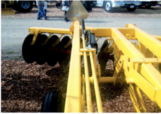
SPLIT AXLES ALLOW REGULATING THE DEPTH OF CUT FOR LEFT OR RIGHT SIDE
