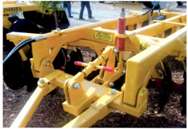
HITCH TURNBUCKLE ALLOWS REGULATING DEPTH OF CUT FOR FRONT OR REAR GANGS
